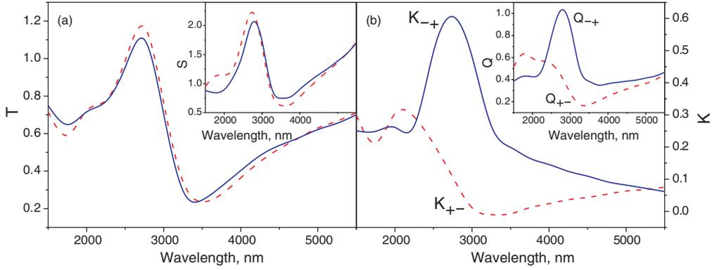
**Figure 3.** Shown are the spectral dependences for a chiral gammadion hole: integral transmission ( $S$ ,  $T$ ) and polarization conversion ( $Q$ ,  $K$ ) for circularly polarized light in terms of the Stokes parameter ( $S$ ,  $Q$ ) and Poynting vector ( $T$ ,  $K$ ) representations. Solid lines correspond to LCP illumination, dashed to RCP.
