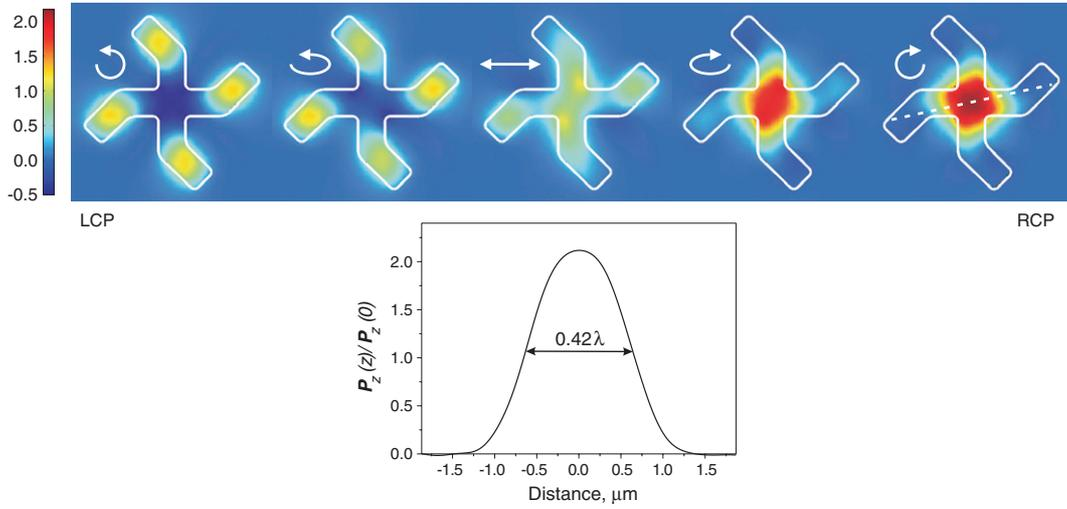
**Figure 4.** The transmitted intensity  $P_z(\mathbf{r}, z)/P_z(\mathbf{r}, 0)$  behind the gammadion hole depends on the polarization state of the incident light, as indicated by adjacent arrows. Below is an intensity profile plot, which was taken along the direction indicated by the dashed line on the field map to the far right for RCP illumination.
